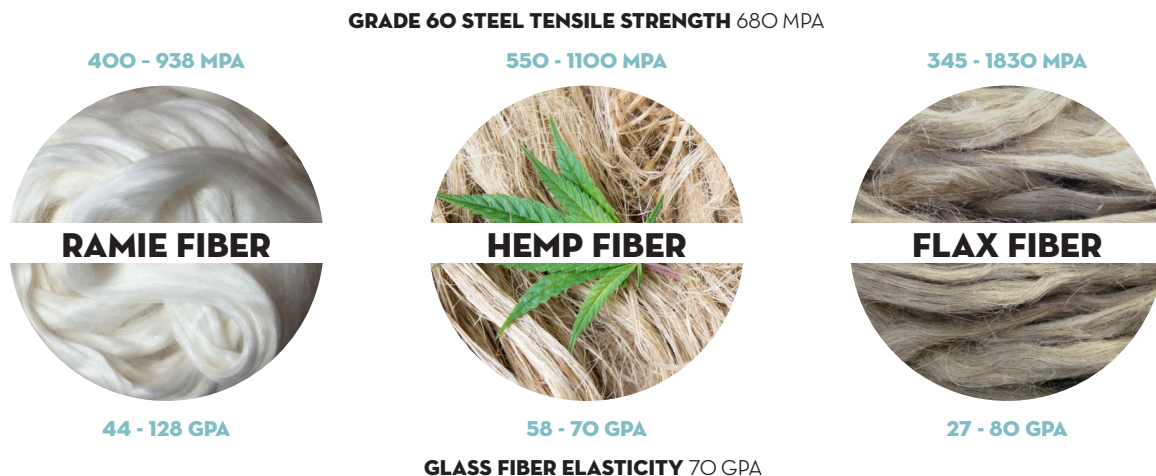
Figure 2. Mechanical properties of various natural fibers. Daniel M. Cohen M.Sc., RA, LEED AP.
